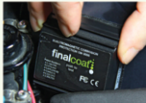
Final Coat’s industry-leading CM-3000 module only draws 0.3 milliamps.
